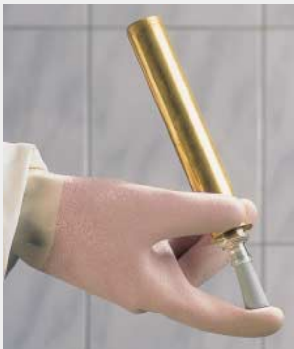
The butyrometer in the casing is shaken (goggles and rubber gloves must be worn).
