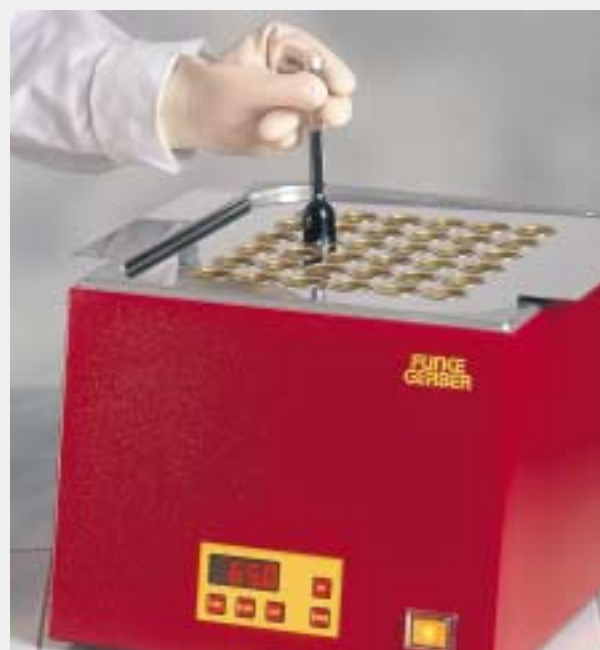
The butyrometers are brought to the exact read-off temperature in the water bath.
