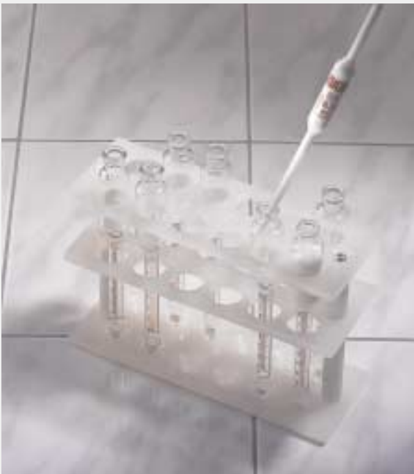
10,75 ml of milk are pipetted into the butyrometer.
