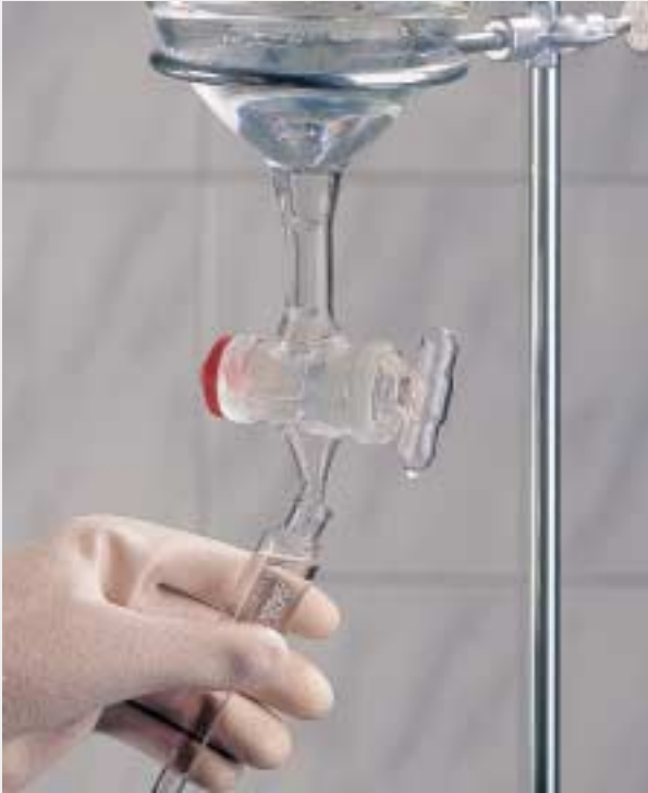
When filling with sulphuric acid make sure you wear goggles and rubber gloves.
